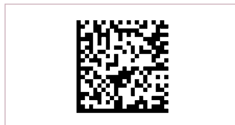
Image 7: Example of a GS1 Data Matrix code
